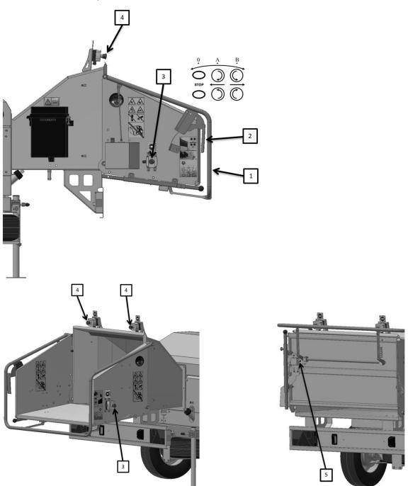
The wood chipper is equipped with TP E-STOP, which consists of four emergency stop buttons (3) and (4). An emergency stop button (3) is fitted on each side of the funnel, and two emergency stop buttons (4) are fitted above the funnel. They are all controlled by a control box based on a sensor (5) on the safety bar (1) with a reset handle (2). (See illustration above).
