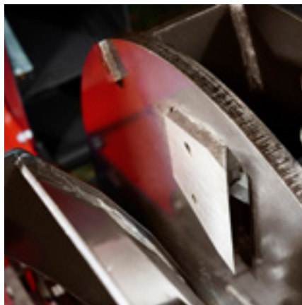
Displaced blades (2 pcs.) constantly engaging material
