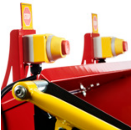
TP E-STOP is standard for operator safety
