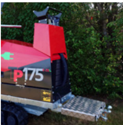
Manual control panel and platform with 44 lb safety switch
