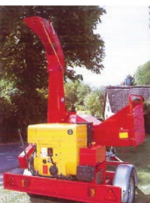
Mobile wood chipper with own motor Trailer-based models have gained ever-greater market share since the mid-1990s.
