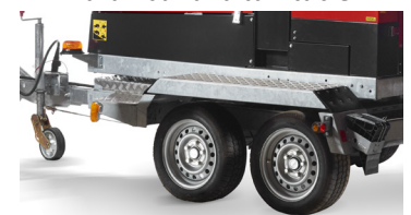
Twin axle trailer with fixed drawbar and turntable
