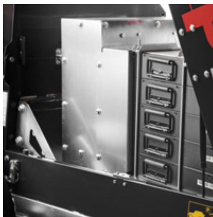
21 kWh De lithiumbatterij (Li-ion, 65VDC, NMC)
